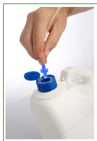
Figure 5: Open the bottle cap and press the Blue quick connect into the opening on the bottle.
